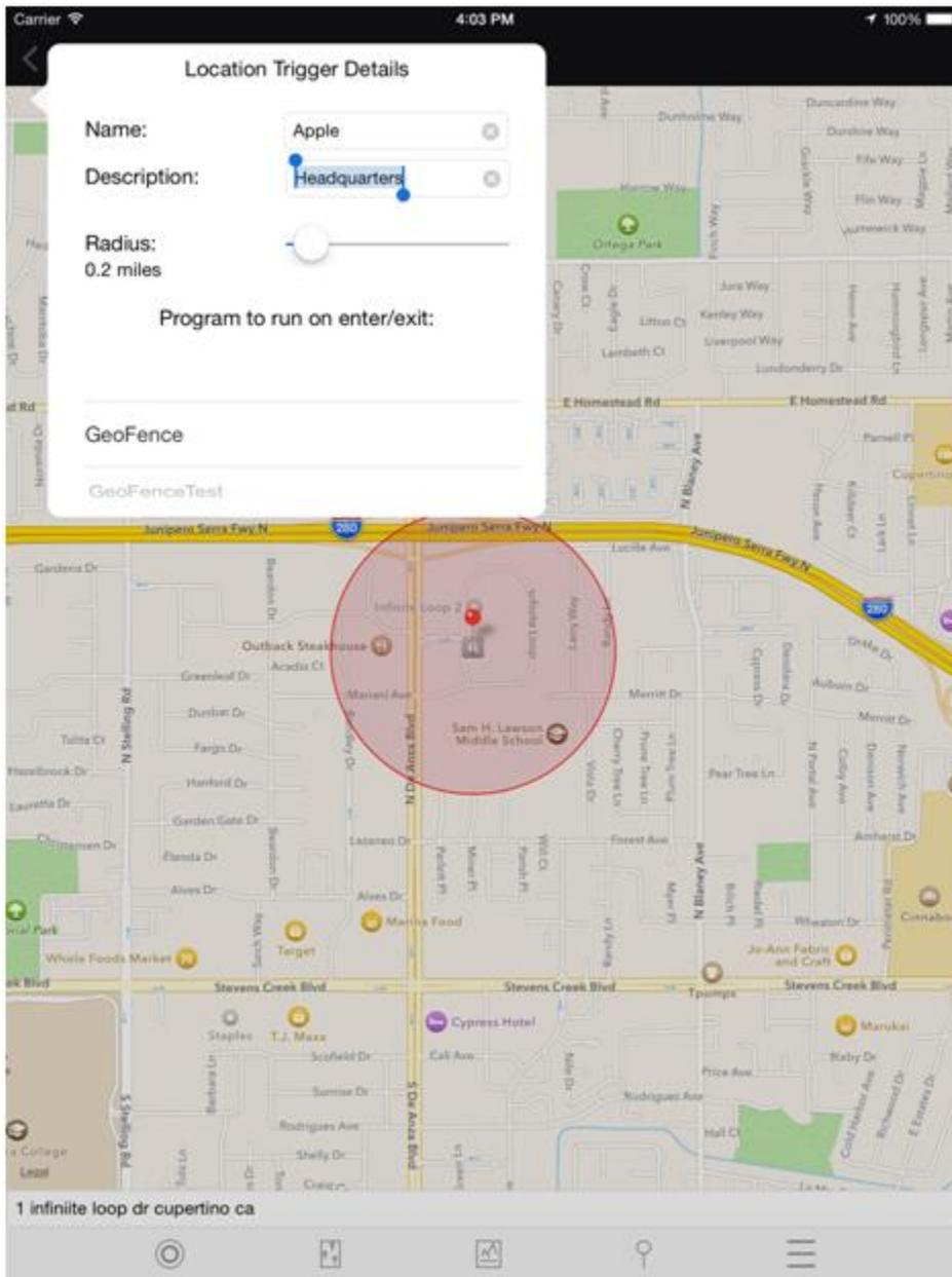
Enter a name for this Geofence – it is passed to the associated HCA Program when that program is started, a description – also passed as an argument to the program, the radius of the fenced area, and the name of the HCA program to run when entering or exiting the area. Only the programs in the “Location Aware Programs” folder are available for selection.
