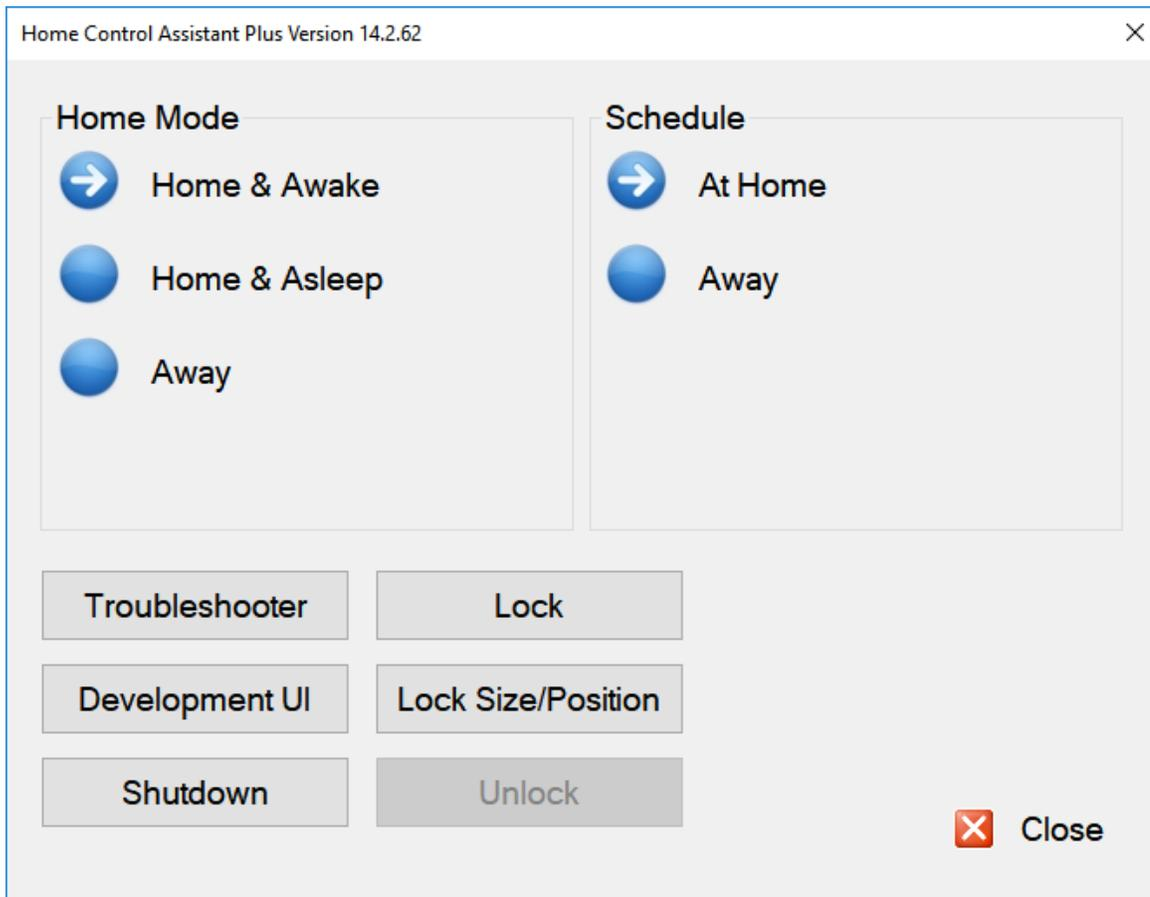
In the control panel you can return to the Development UI by pressing the button labeled for that. Also in the control panel you can change the current Home Mode and schedule.
